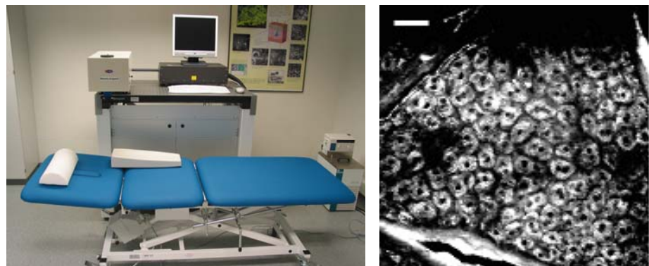
Figure 2. Left panel: "Dermalinspect" system (box on the left of the optical table) with a pulsed femtosecond laser (box on the right of the optical table), and with a bedside. Right panel: MPM imaging of the epidermis layer of live skin. Note clearly resolved cells and cell nuclei. Scale bar, 20\ \mu\text{m} . (Courtesy of Prof König, JenLab, Inc.)
