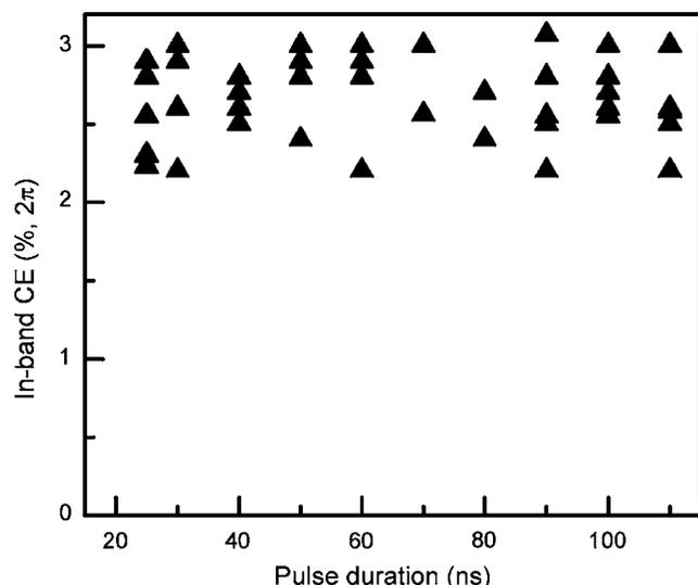
FIG. 2. In-band CE from CO<sub>2</sub> laser-produced Sn plasma as a function of laser pulse duration.
