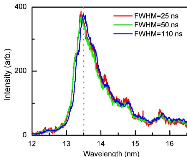
FIG. 3. (Color online) Soft x-ray spectra obtained with various laser pulse durations of 25 (red), 50 (green), and 110 ns (blue).
