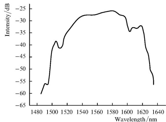
Figure 5. Emission spectrum of the master oscillator.
