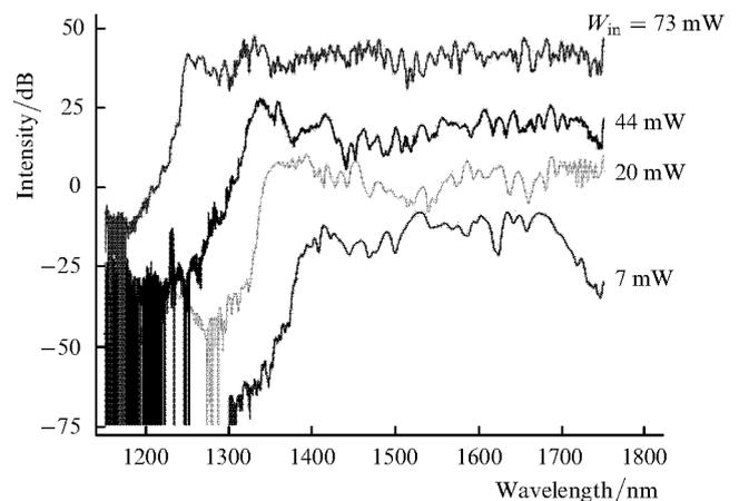
**Figure 8.** Dependence of the supercontinuum spectrum on the average radiation power  $W_{\text{in}}$  coupled into fibre IV with a high nonlinearity and shifted dispersion.
