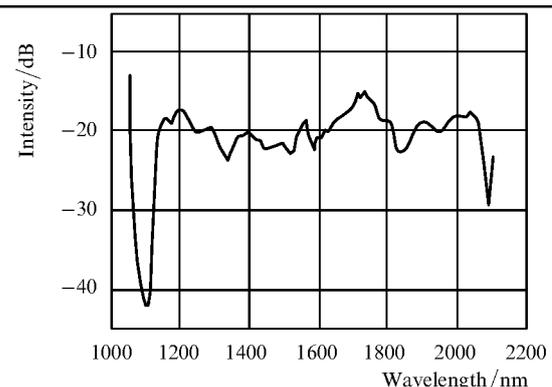
**Figure 9.** Long-wavelength part of the supercontinuum spectrum.
