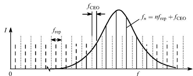
**Figure 1.** Scheme of the frequencies of a cw femtosecond laser (solid straight lines), the same frequencies attached to the coordinate origin (dashed straight line), and equidistant frequencies with the same period (dotted straight lines);  $f_{\text{rep}}$  is the intermode interval,  $f_{\text{CEO}}$  is the carrier frequency-envelope maximum offset, and  $f_n$  is the frequency of the  $n$ th mode.
