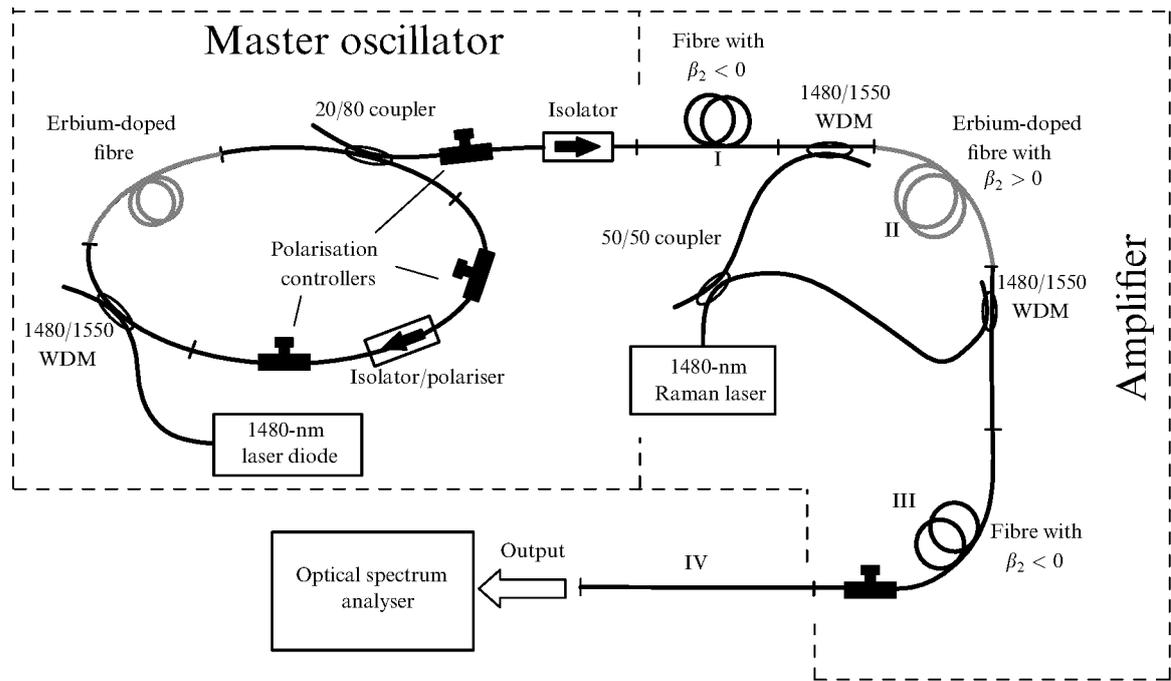
Figure 3. Scheme of the master oscillator–amplifier setup.
