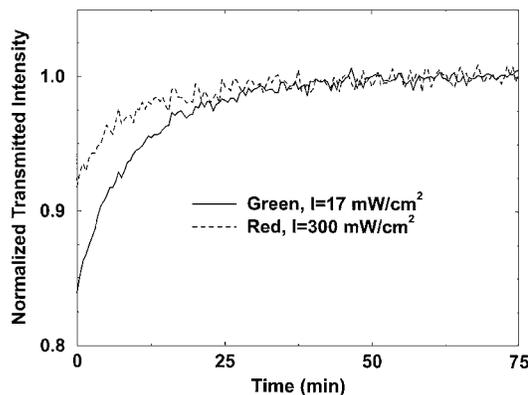
Fig. 3. Normalized intensity of transmitted light for bleaching experiments with a 0.85-mm-thick, UV-preexposed  $\text{LiNbO}_3\text{:Fe:Mn}$  crystal.
