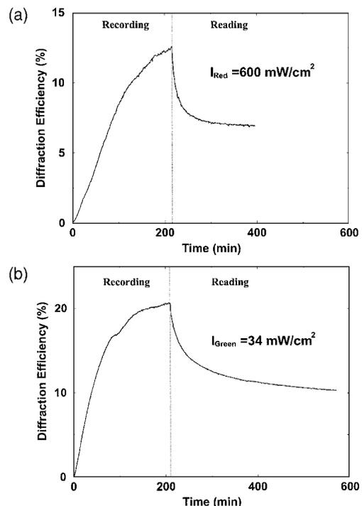
Fig. 1. Recording and readout curves for a plane-wave hologram in a 0.85-mm-thick LiNbO<sub>3</sub>:Fe:Mn crystal. Recording was performed by simultaneous presence of a homogeneous UV beam and (a) two red beams or (b) two green beams.
