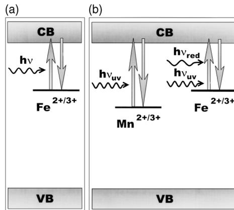
Fig. 2. Energy-band diagrams for a typical  $\text{LiNbO}_3$  crystal doped with (a) Fe or (b) Fe and Mn. CB, conduction band; VB, valence band.
