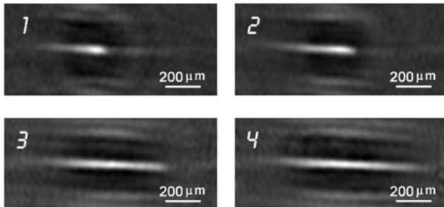
Fig. 5. Instantaneous time evolution of the electron density. The relative time of the snapshots is  $t_1 = 0$ ,  $t_2 = 1 \text{ ps}$ ,  $t_3 = 2 \text{ ps}$ , and  $t_4 = 2.7 \text{ ps}$ . Because of the small angular aperture, fine structure is not recovered.
