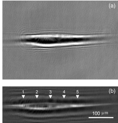
Fig. 2. (a) In-line hologram of the plasma distribution. The image resolution is  $2184 \times 1472$ , and the pixel size is  $6.8 \mu\text{m} \times 6.8 \mu\text{m}$ . The hologram is captured at  $L = 30 \text{ cm}$  with a magnification of  $M = 12.5$ . (b) Spatially resolved electron density calculated from the phase change.
