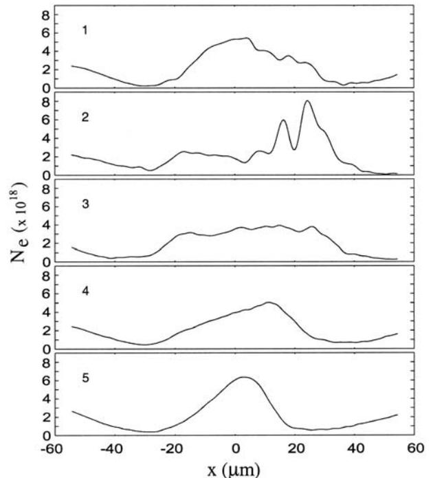
Fig. 3. Electron density distribution at various cross sections showing detailed plasma evolution. Distances from the onset of the plasma are 1, 326  $\mu\text{m}$ ; 2, 435  $\mu\text{m}$ ; 3, 544  $\mu\text{m}$ ; 4, 652  $\mu\text{m}$ ; 5, 761  $\mu\text{m}$ .
