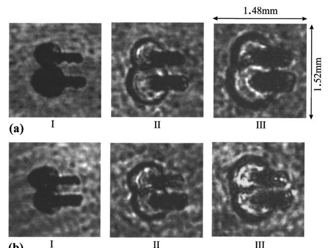
FIG. 3. Interaction of two shock waves. (a) Unbalanced double shock waves. (b) Equal intensity waves.
