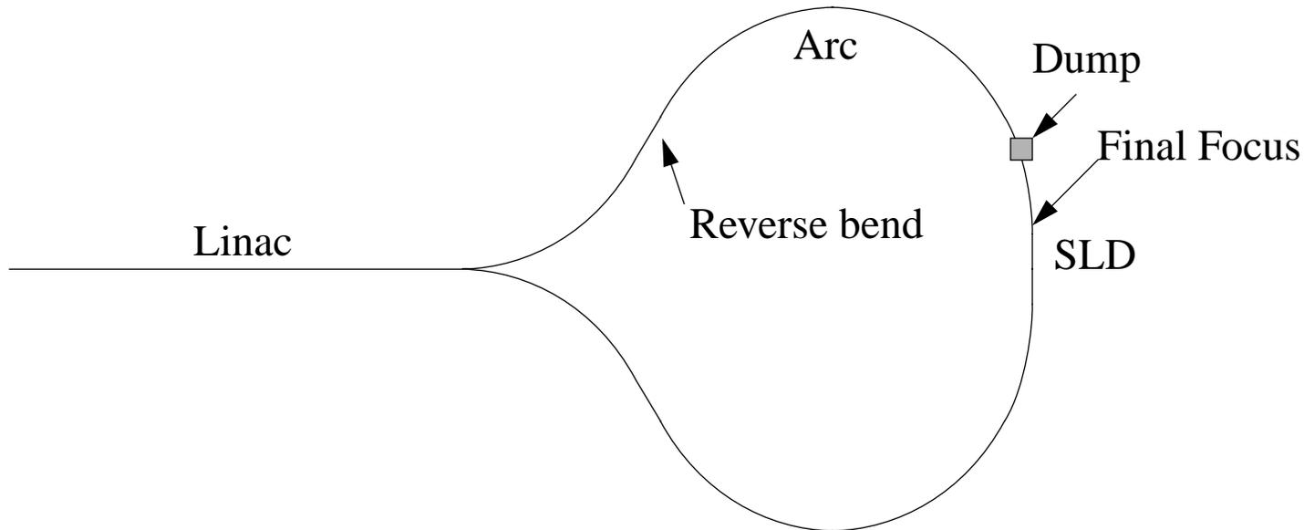
Simulations indicate that short bunches can be produced anywhere between the Reverse bend and the Final Focus. So far, the shortest simulated bunches have been in the Reverse bend region. Bunch lengths of  $\sigma_z < 50\mu\text{m}$  are also possible in the Final Focus area.
