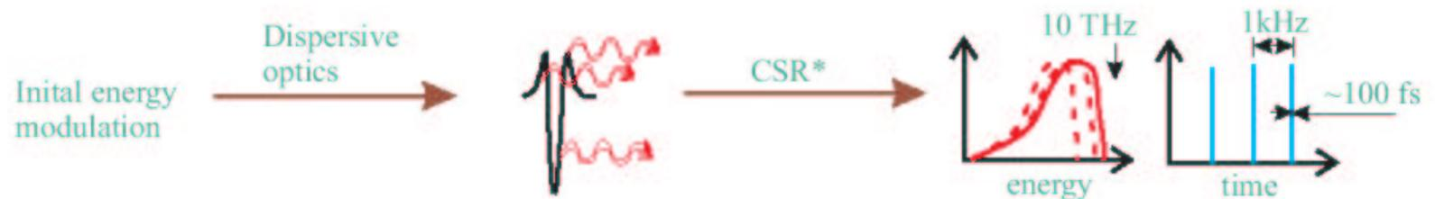
Sliced electrons ( $\simeq 100$  fs) and dip in the bunch emit **coherent** radiation ( $\propto N_e^2$ );
