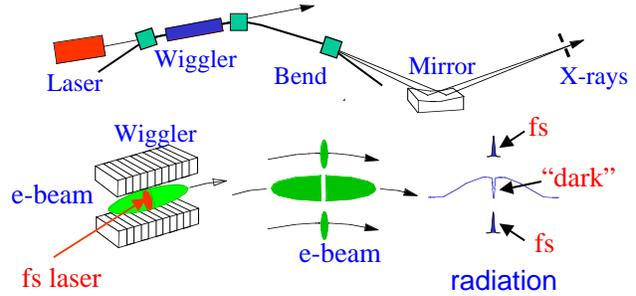
Figure 1: A schematic of generation of the femtosecond pulses of synchrotron radiation.
