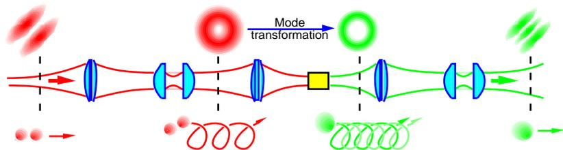
wave fronts associated with LG modes imply that the Poynting vector follows a spiral path as it propagates<sup>7</sup>. In isotropic media the wave vector follow the same path as the Poynting vector. Consequently, these findings led us to consider the behaviour of LG modes within nonlinear optical interactions. When a LG mode is frequency doubled, the we found that a mode transformation occurs, doubling the azimuthal index of the mode.
