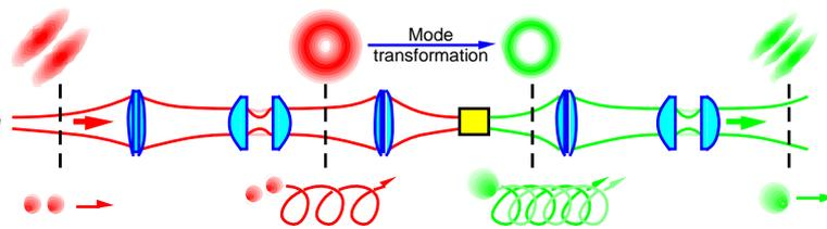
Other "blue-sky" research funded under this grant includes the identification and generation of a class of astigmatic beams which contain orbital angular momentum of many 100's of  $\hbar$  per photon<sup>5</sup> and a new method for the generation of Laguerre-Gaussian laser modes using a stressed fibre optic waveguide<sup>6</sup>.
