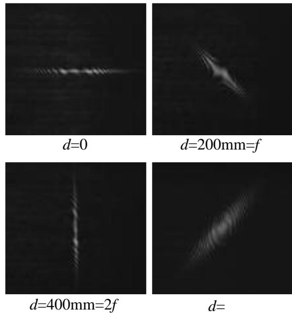
For highly elliptical beams a few millimetres in size, at optical wavelengths, this can easily exceed  $10,000\hbar$  per photon. Only the  $f$ -number and aperture of the cylindrical lens limits the amount of orbital angular momentum that can be transferred. It is worth noting that, unlike the Laguerre-Gaussian beams, the elliptical beams have an on-axis intensity.
