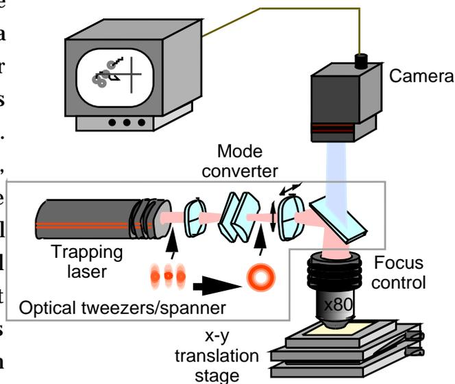
We demonstrated that the *LG* mode produces a stronger tweezers force than the fundamental Gaussian mode used previously. For a wide range of particle sizes the laser power required with an  $\ell = 3$  Laguerre-Gaussian mode is reduced by a factor of two<sup>5</sup>. This is important for biological applications where reduction of the laser power lessens the risk of damage to the living sample.
