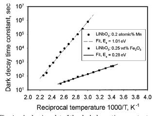
Fig. 4. Arrhenius plot of the dark decay time constants of nonfixed holograms stored in Mn-doped LiNbO<sub>3</sub> (0.2-at. % Mn), and Fe-doped LiNbO<sub>3</sub> (0.25-wt.%  $Fe_2O_3$ ).
