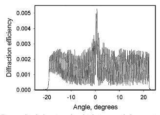
Fig. 2. Comb function of multiplexing 100 holograms in  $LiNbO_3:0.2$ -at. % Mn. The M/# calculated from this comb function is 5.
