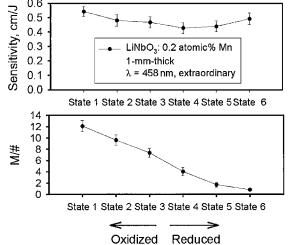
Fig. 3. Measured sensitivity and M/# versus oxidation state in 1-mm-thick LiNbO<sub>3</sub>:0.2 at. % Mn.
