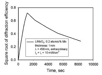
Fig. 1. Typical recording and erasure curve for 1-mm-thick LiNbO<sub>3</sub>:0.2-at. % Mn.
