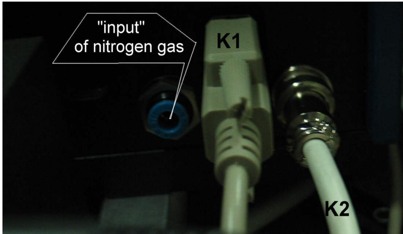
Figure 3.6: Cables connection and “nitrogen” on laser box.
