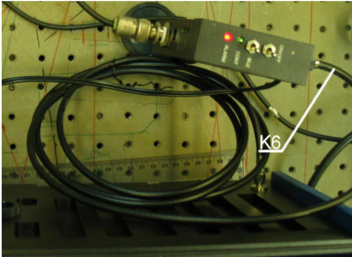
Figure 3.7: Cables connection of Electrical Starter with laser box.
