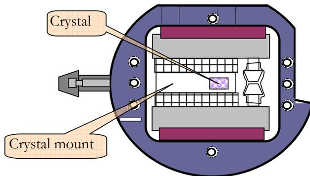
*Figure 1.1: Interior of crystal housing.*
