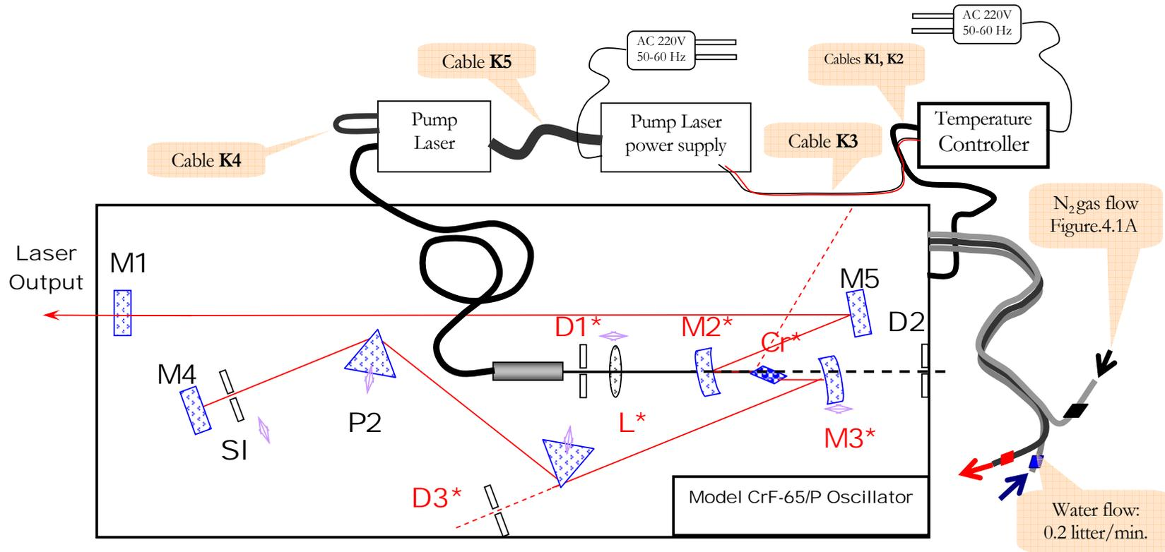
Figure 3.3: Cable and tube connections for CrF-65/P model Femtosecond Forsterite Laser.
