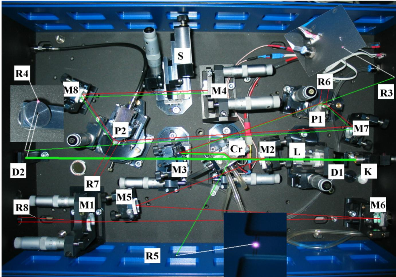
Figure 4.15: Schematic for CrF-65/P model Femtosecond Forsterite Oscillator. Green beam – pump, red beam – radiation at 1250nm
