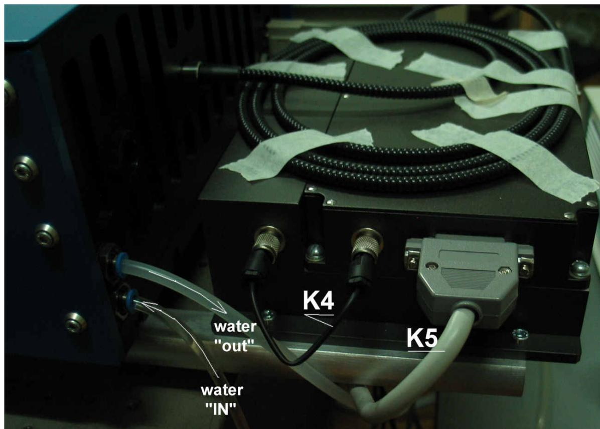
Figure 3.5: Cables connection on Pump laser and water flow direction on laser box.
