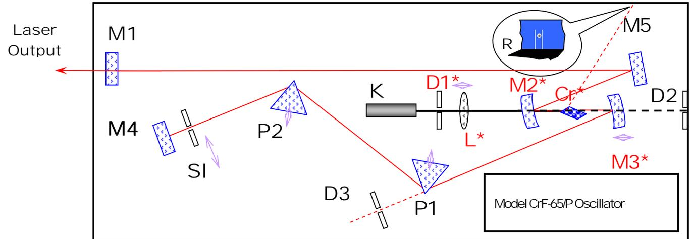
Figure 4.14: Schematic for CrF-65/P model Femtosecond Forsterite Oscillator: Mirrors M6-M8 are not shown on the picture.
