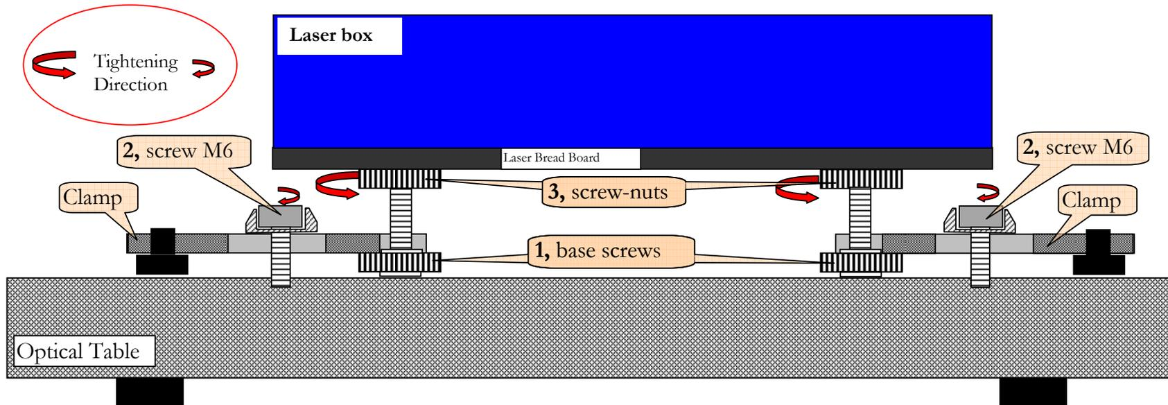
Figure 3.1. Schematic for mounting laser system on optical table.
