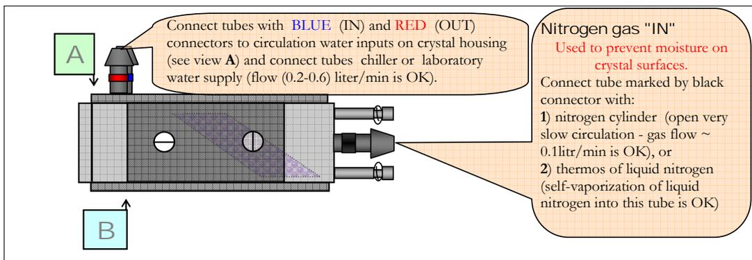
Figure 3.2: Schematic picture of Crystal housing. Note: Please see Figure 7 for Views **A** and **B**. (In laser head the bottom pipe is **BLUE** (water “IN”) and top pipe is **RED** (water “OUT”))
