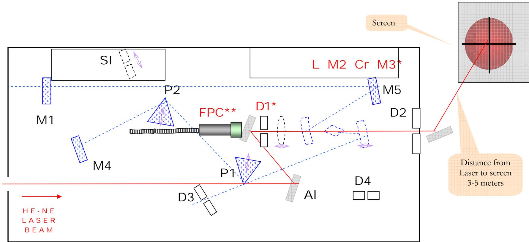
Figure 5.1 Oscillator cavity alignment using He-Ne laser.
