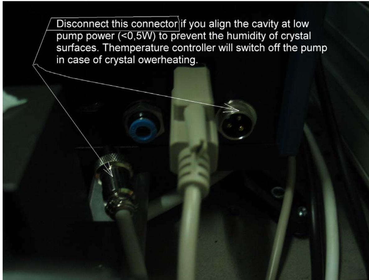
Figure 3.8: Laser operation at low (<math><50\text{mW}</math>) pump power.
