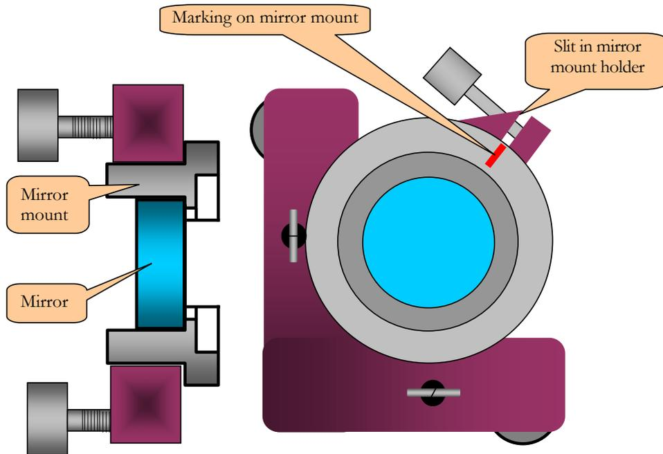
Figure 4.4: Schematic picture of Mirror mount assembly.
