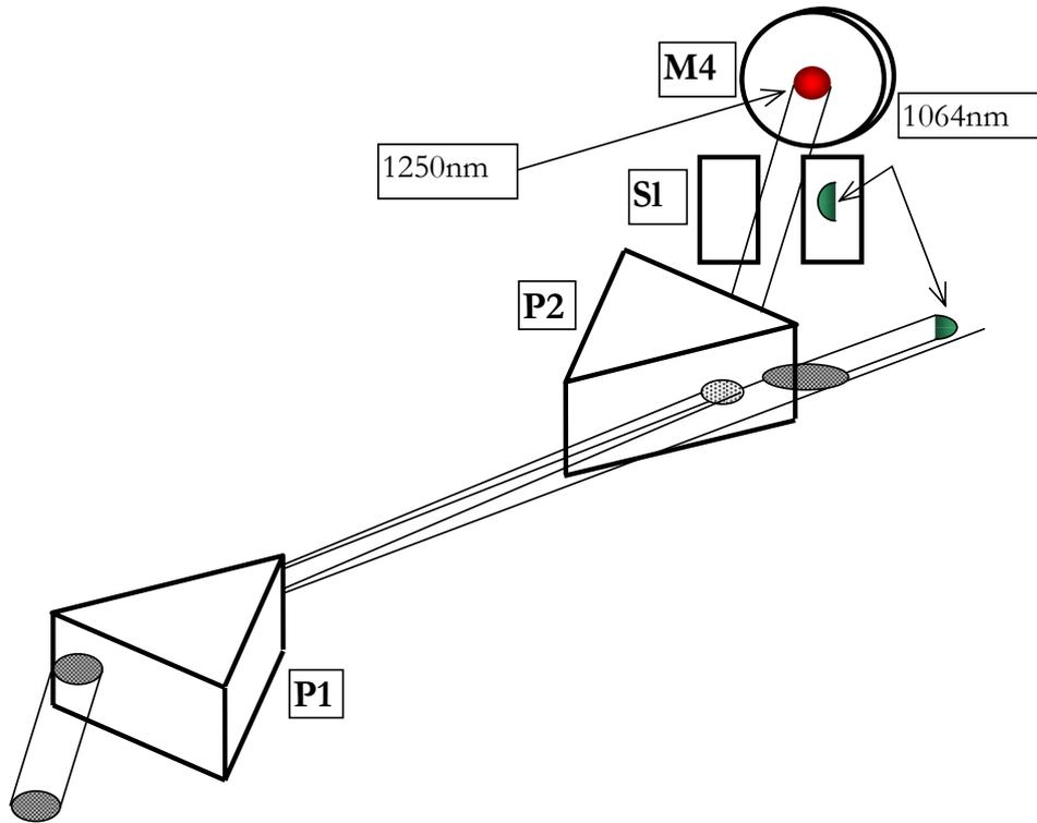
Figure 6.5. Beam positions on prisms and slit.
