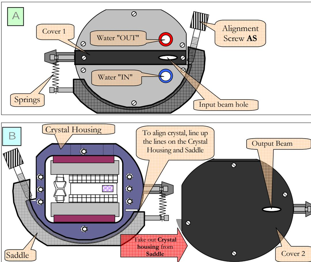
Figure 4.1: Front and back views of the Crystal housing.
