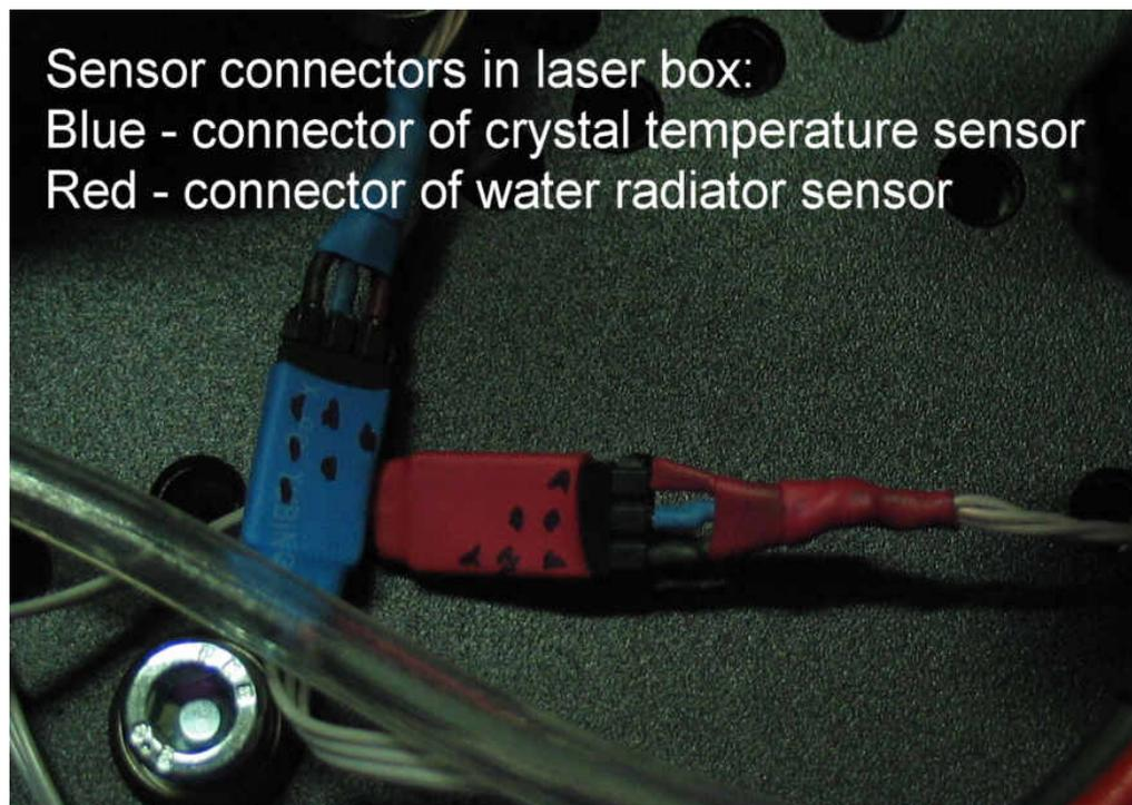
*Figure 3.10: Sensors connections in laser box*
