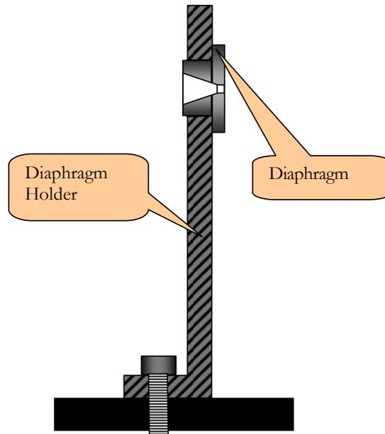
Figure 4.5: Schematic of Diaphragm and holder.
