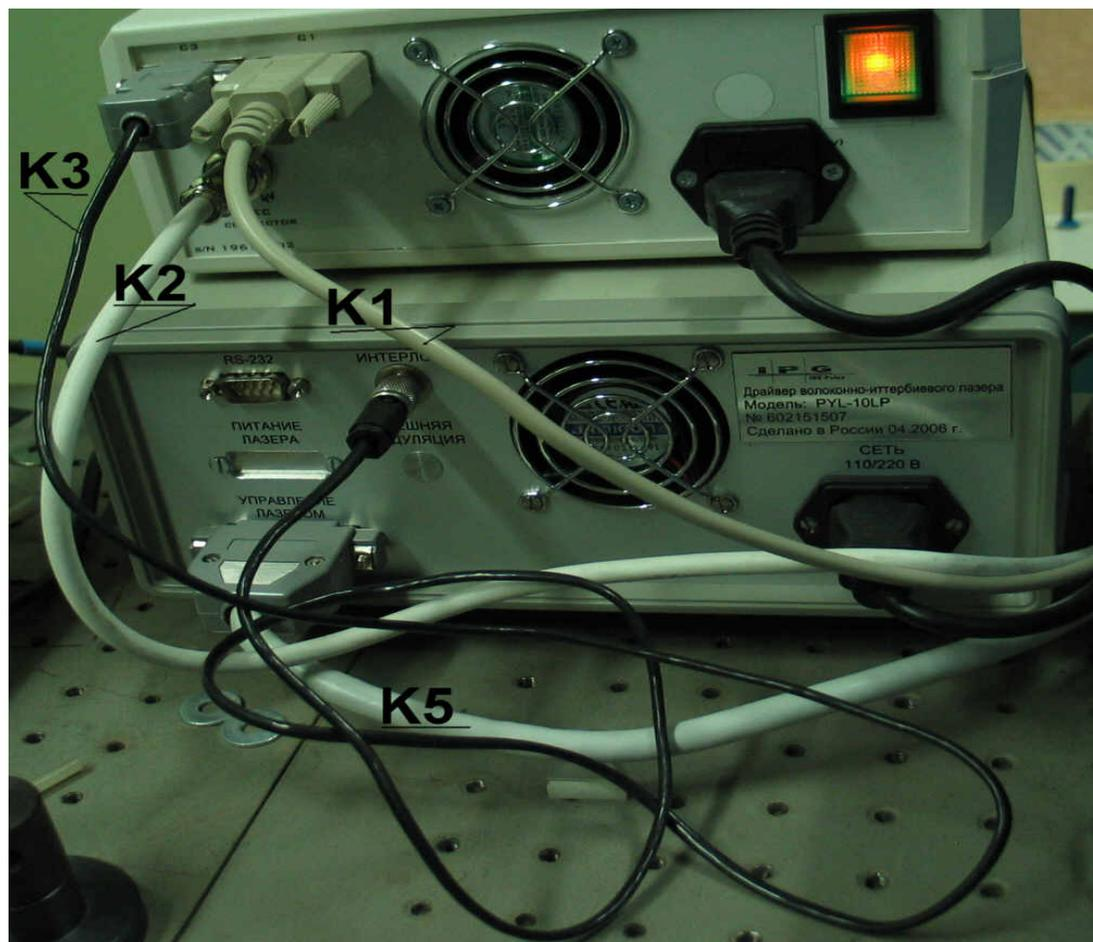
Figure 3.4: Cables connection on Power Supply of Pump laser and on Temperature controller
