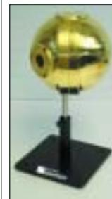
A series of integrating spheres with electrochemically plated gold surfaces is available from SphereOptics, based in the US. The company claims that its ZenithGold-plated surfaces exhibit diffuse reflectance values of approximately 94–96% over
