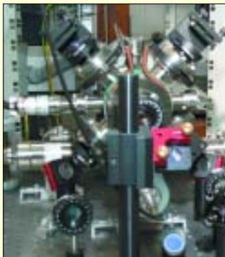
A magneto-optical trap in the cold-atom facility of Poland's National Laboratory of AMO Physics.
