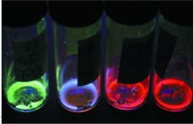
Quantum-dot coding: dots with different emission colours can be combined to create a unique identification label. The invention could put an end to barcodes.
