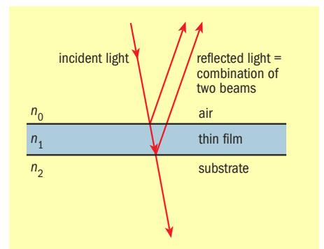
**The principle of a thin-film coating:** interference between reflections from a single film (above) or multiple layers (left) determines the precise optical characteristics of a particular coating.
