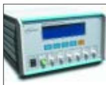
id Quantique, the Swiss start-up that is a specialist in quantum cryptography, has developed a single-photon detector
