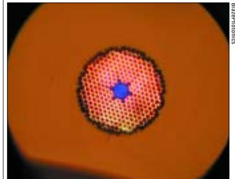
**Ahead of the rest: photonic-crystal fibre is the most commercialized photonic-bandgap technology.**
