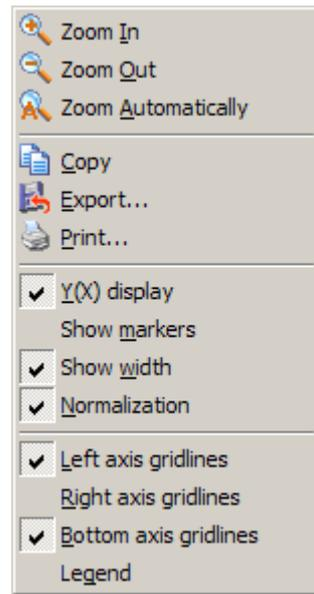
You use Zoom In and Zoom Out menu commands to change the chart display magnification. The command Zoom Automatically restores the chart display magnification to cover the entire data range.
