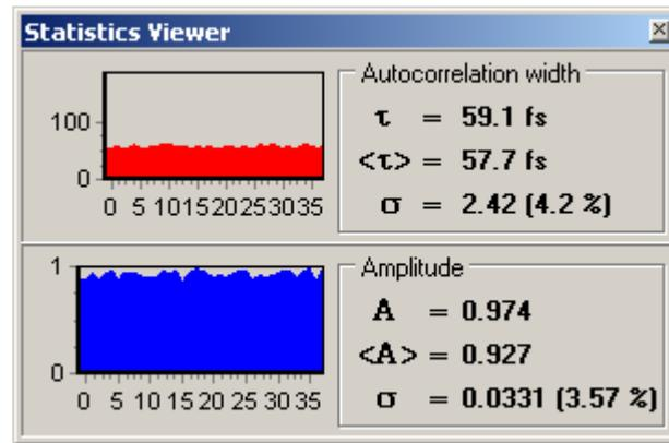
The top pane of the window displays autocorrelation width statistics information. The bottom pane displays amplitude statistics information.
