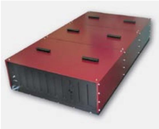
Teahupoo Rider is a fully-integrated all-in-one-box system that includes Trestles Mini Ti:Sapphire oscillator or Buccaneer SHG diode-pumped fiber oscillator, pulse stretcher, regenerative amplifier pumped by multi kHz Nd:YAG pump laser and pulse compressor. Teahupoo Rider has a factory preinstalled repetition rate of 2, 5 or 10 kHz and ideal for low cost femtosecond micromachining systems, OPA pumping, ultrafast spectroscopy and variety of applications in life sciences.
