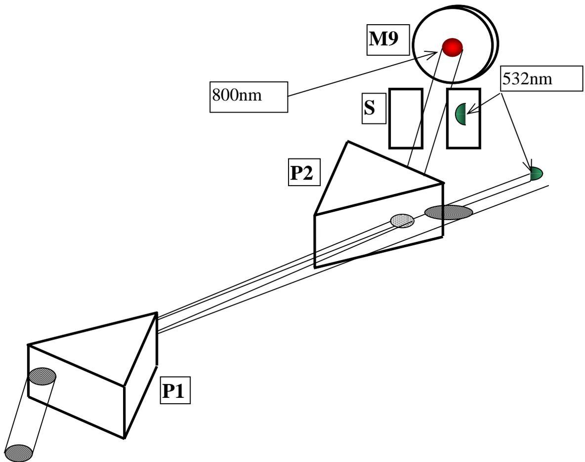
**Figure 10. Beam positions on prisms and slit.**
