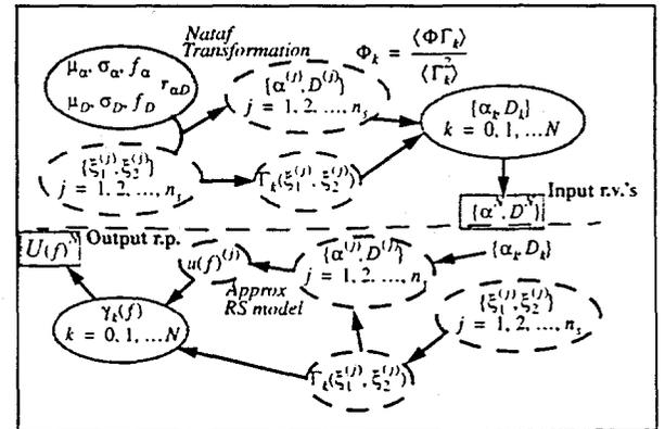
Figure 7: Algorithm used to apply the PCE.
