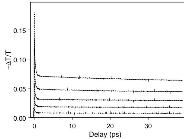
**Figure 2.** Time-resolved negative differential transmittance of a nc-Si:H thin film with dilution ratio  $R = 5$ . The data traces correspond to initial carrier densities of approximately  $1.5 \times 10^{19} \text{ cm}^{-3}$ ,  $1.2 \times 10^{19} \text{ cm}^{-3}$ ,  $9.0 \times 10^{18} \text{ cm}^{-3}$ ,  $6.0 \times 10^{18} \text{ cm}^{-3}$ , and  $3.0 \times 10^{18} \text{ cm}^{-3}$ . The solid lines correspond to fits to the multi-component model described in the text.
