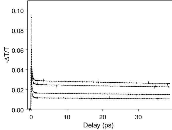
**Figure 3.** Time-resolved negative differential transmittance of a nc-Si:H thin film with dilution ratio  $R = 10$ . The data traces correspond to initial carrier densities of approximately  $1.8 \times 10^{19} \text{ cm}^{-3}$ ,  $1.5 \times 10^{19} \text{ cm}^{-3}$ ,  $1.2 \times 10^{19} \text{ cm}^{-3}$ , and  $9.0 \times 10^{18} \text{ cm}^{-3}$ . The solid lines correspond to fits to the multi-component model described in the text.
