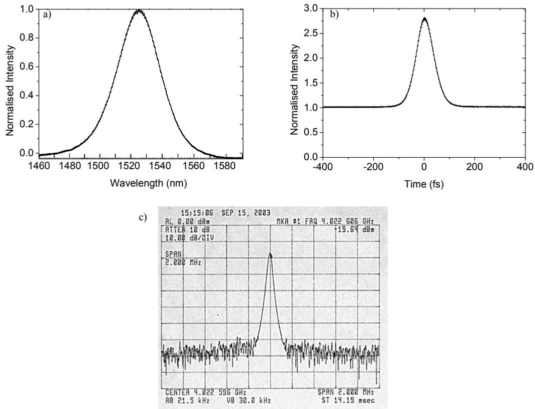
Figure 2 a) Spectral trace, b) Autocorrelation and c) Frequency trace of laser running at 4.02 GHz
