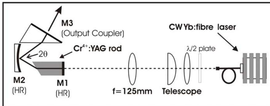
Figure 1. Schematic diagram of KLM Cr<sup>4+</sup>:YAG laser
