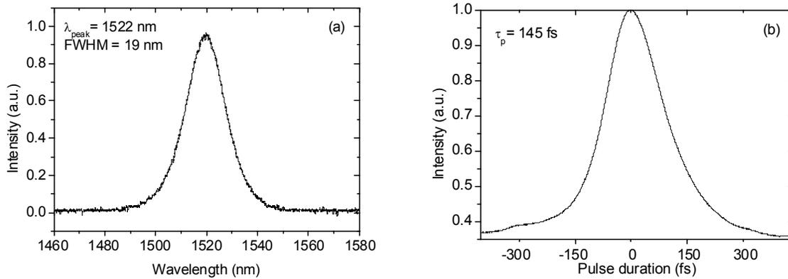
Figure 2. Optical spectrum (a) and intensity autocorrelation (b) of femtosecond pulses from a  $\text{Cr}^{4+}$ :YAG laser at a prf of 3.4 GHz.
