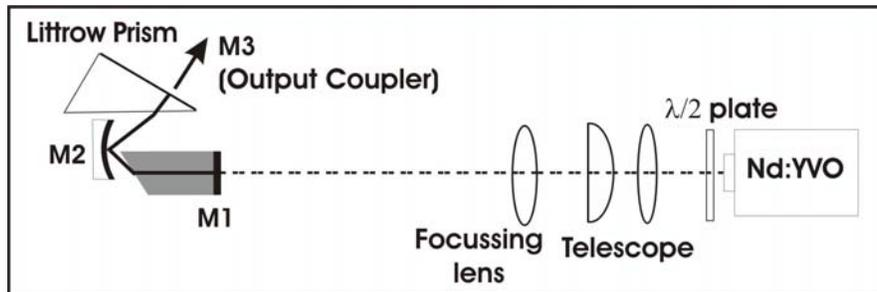
Figure 1. Schematic diagram of KLM Cr<sup>4+</sup>:YAG laser
