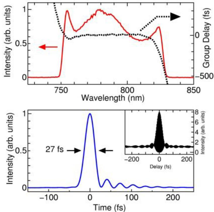
Fig. 4. Spectral intensity and phase, based on a SPIDER measurement (above).
