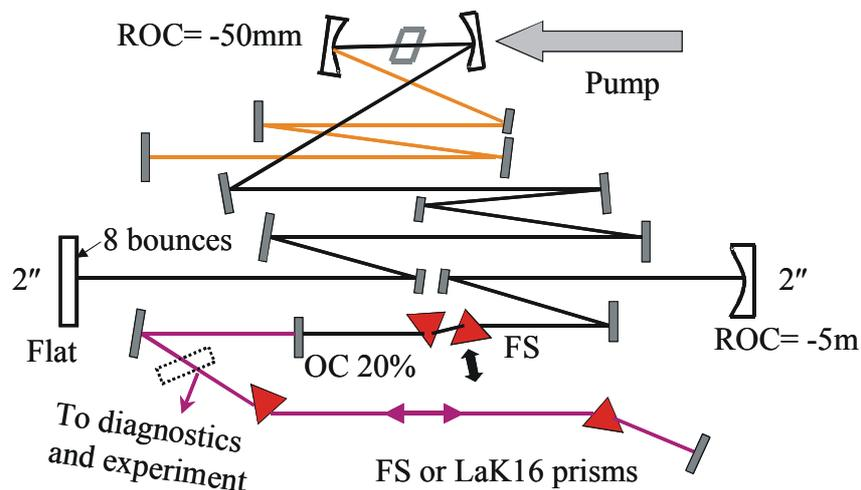
Fig. 1. Experimental Setup of the extended cavity oscillator
