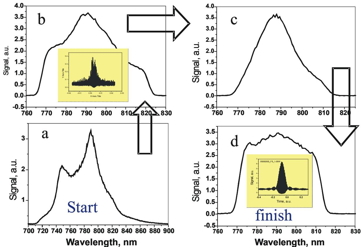
Fig. 2. Evolution of the spectral intensity for an increasing amount of net-GDD inside the cavity.
