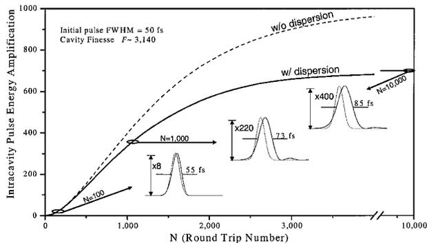
Fig. 4. Results from time-dependent calculation showing the coherent evolution of a 50-fs pulse inside the cavity. Dashed curve, ideal case of a dispersion-free cavity perfectly matched with the incident pulse train; solid curve, effect of cavity dispersion in limiting the amount of energy coupled into the cavity.
