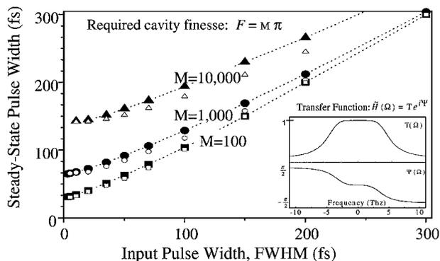
Fig. 2. Relationship between input and output (amplified) pulse widths through the cavity for three maximum cavity magnifications ( $M$ ). Filled (open) points indicate results from steady-state (time-dependent) calculations. Inset, transmission and phase coefficients of the cavity transfer function for the pulse train obtained from steady-state calculations. Even for an amplification factor of 1000, output pulses well under 100 fs are achievable.
