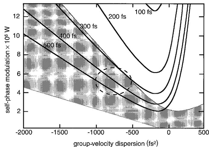
**Fig. 3. Theoretical stability region (shaded area). The operating region of the laser is enclosed by the dashed ellipse.**
