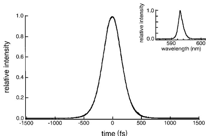
**Fig. 2. Autocorrelation trace of the output pulses at 593 nm and the  $\text{sech}^2$  fitting curve. Inset: the corresponding power spectrum.**
