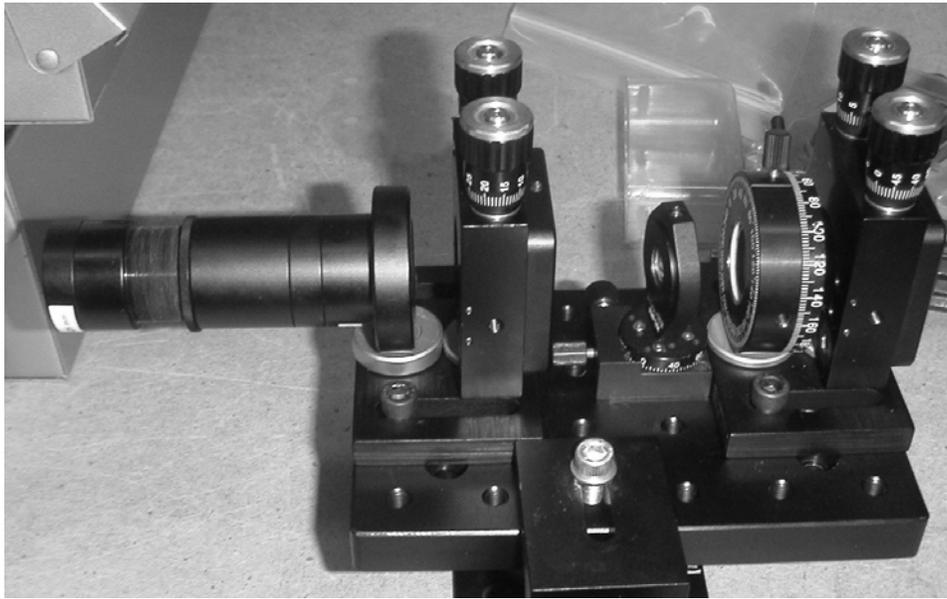
Picture 6.1: Photograph of the finished tripler.
