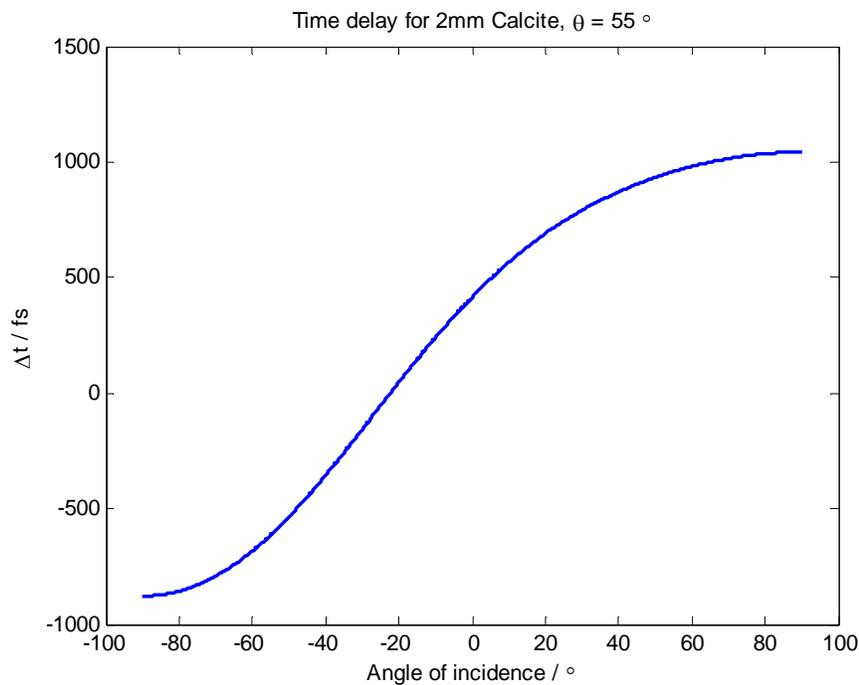
**Figure 3.14: Example curve for a Calcite compensation plate.**
