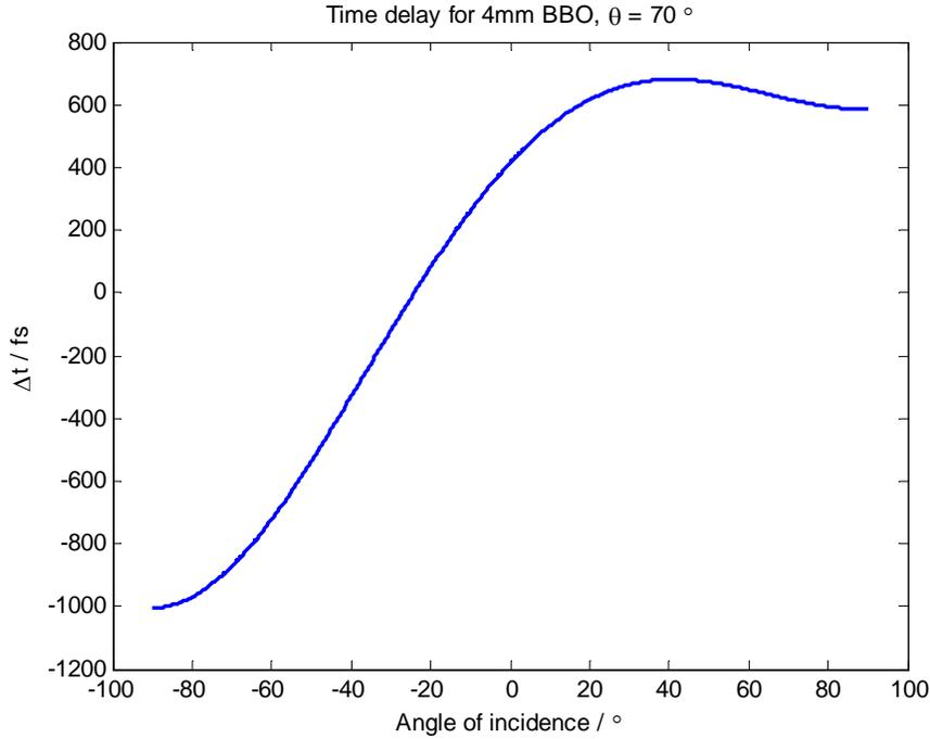
Figure 3.13: Example curve for a BBO compensation plate.
