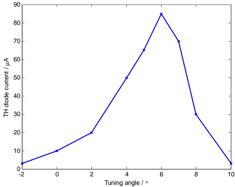
**Figure 5.1: The third harmonic diode current as a function of tuning angle.**
