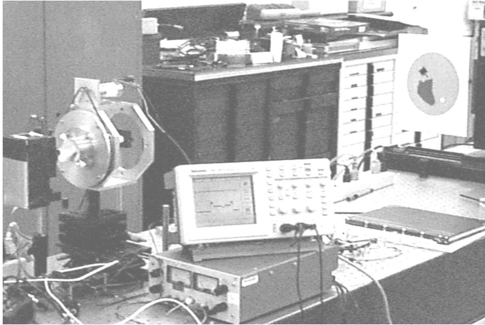
**Figure 3 Visible light prototype seeker on a laboratory test stand.**
