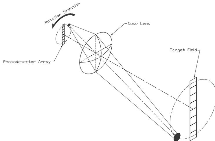
Figure 1 Schematic diagram of seeker concept
