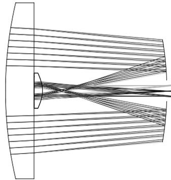
**Figure 2 The compact folded lens uses one aspheric element with two commercially available lenses to produce an effective focal length of 30-mm with a diameter of 25-mm.**
