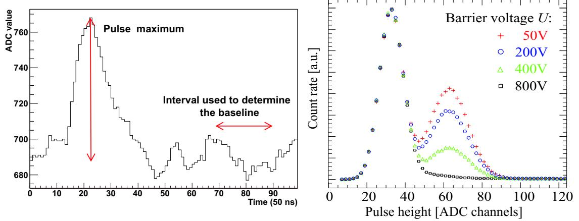
**FIGURE 3.** Left: Pulse shape signal for one event. Here the maximum value of the signal and the interval of time used to determine the baseline (mean value of the interval taken at the tail of the signal) are marked. The difference between them is the proton pulse height. Right: Pulse height spectrum of the proton detector for different barrier voltages  $U$  in the Analyzing Plane. The signal to background ratio is better than 10:1 below the proton peak.
