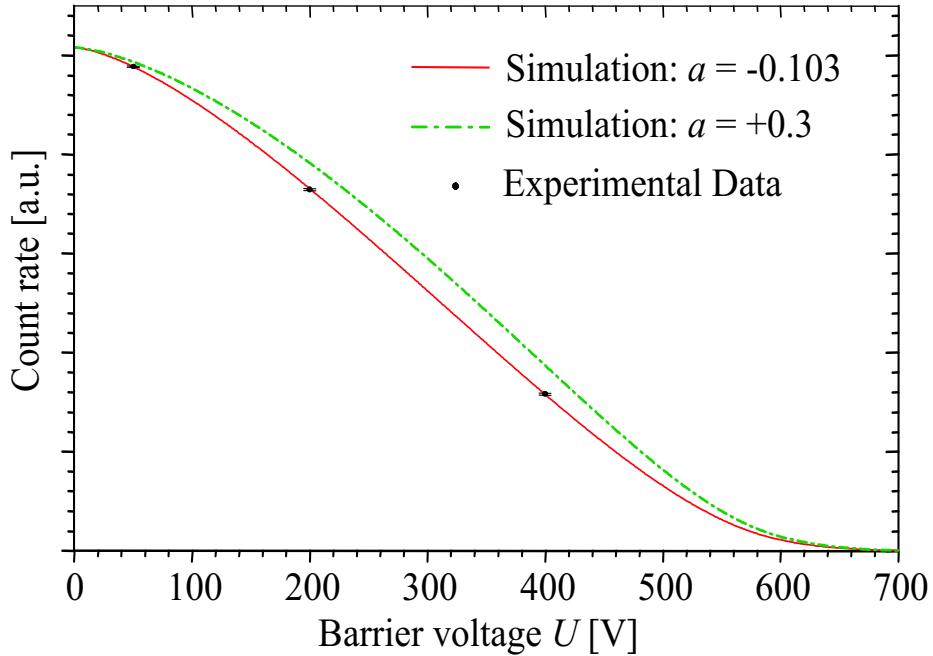
**FIGURE 5.** Total proton count rate vs. barrier voltage after the subtraction of the background. The solid line is the prediction from the Standard Model with the recommended value for  $a$ , the dashed line shows how a deviation from that would look like.
