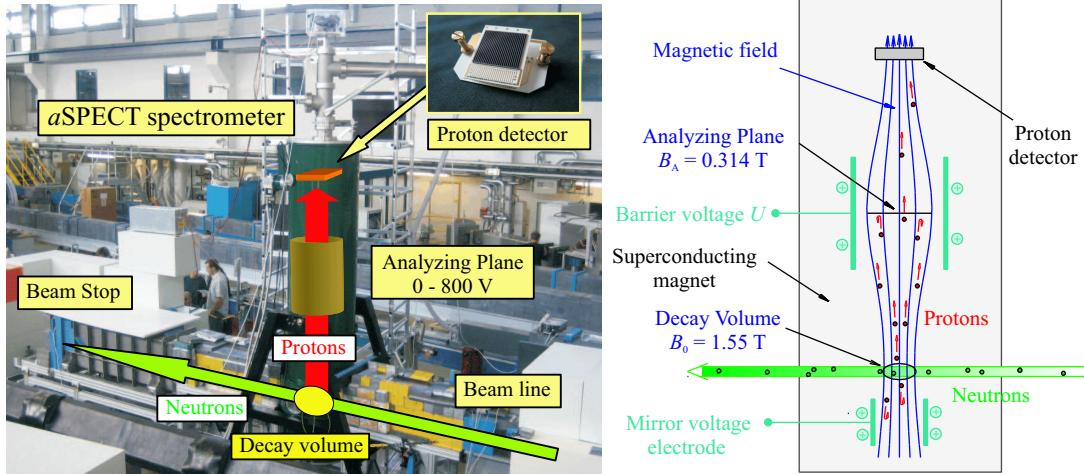
**FIGURE 2.** Setup of the experiment, at the left as a picture, at the right as a sketch. A neutron beam (the green arrow) is guided through the spectrometer. Some neutrons decay in the decay volume, and the decay protons are guided by a magnetic field to the proton detector.
