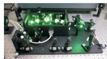
⊙ Fast two-stage system of locking the cavity to the frequency of input radiation
